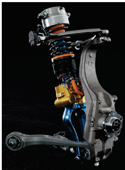
Purosangue front suspension corner. Each TASV damper integrates a liquid-cooled, 48-volt brushless electric motor with dual spool valves that independently manage rebound and compression.
