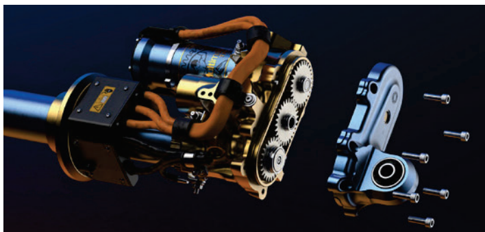
TASV's electric motors apply direct force to the vehicle chassis and damper piston rods through a ball-screw and worm-gear assembly.
