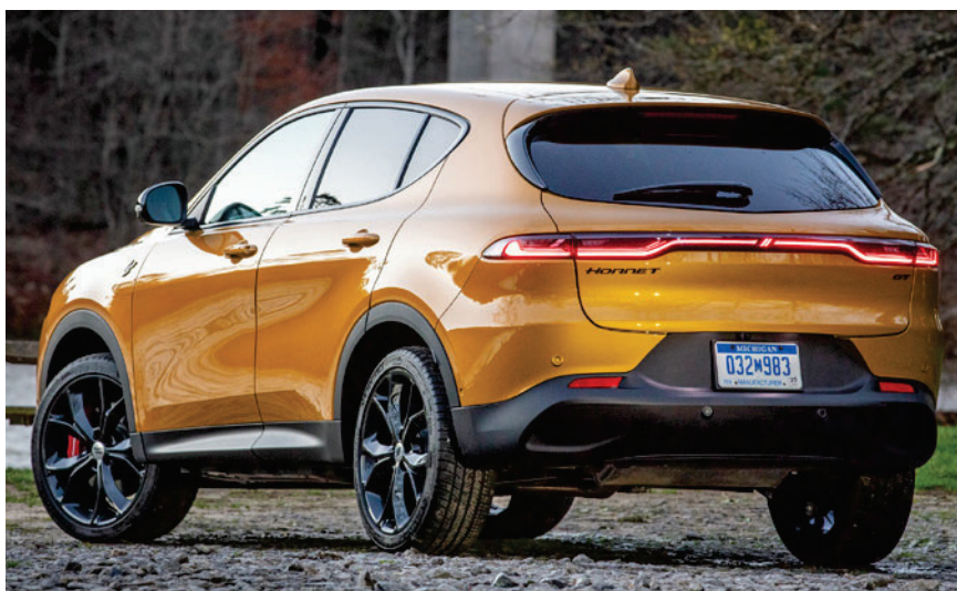
The 2024 Hornet R/T is a plug-in hybrid that couples a 1.3L 4-cyl. with a starter-generator motor and a rear e-axle.
